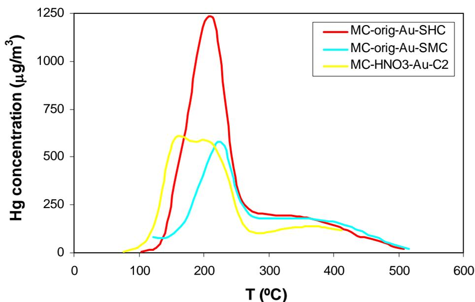
Figure 7. Hg temperature programmed desorption for exhausted sorbents
