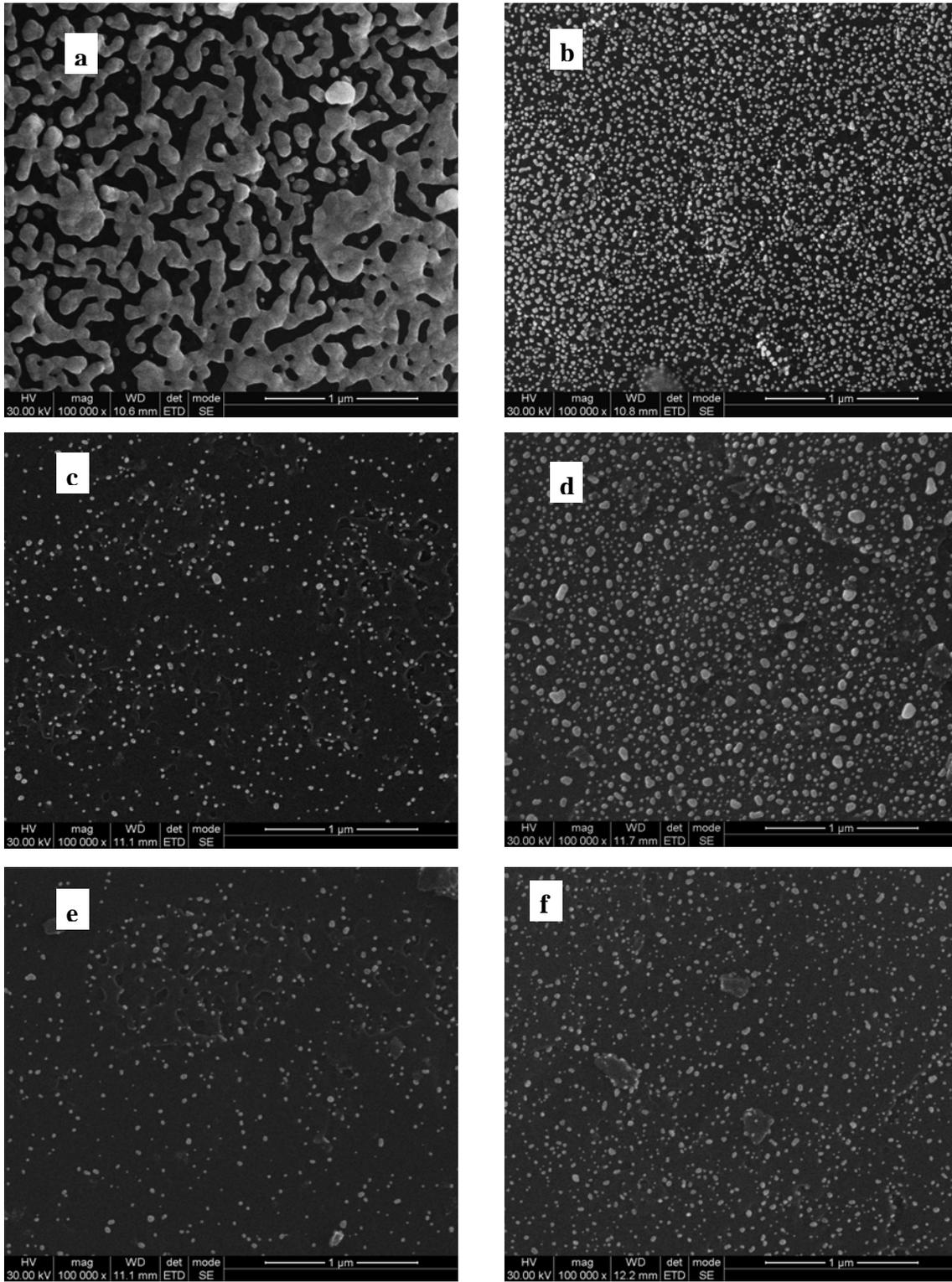
Figure 2. Fe-SEM micrographs of the sorbents, Au particle size distribution and circularity of the Au particles : a) MC-orig-Au-HC; b) MC-orig-Au-SMC; c) MC-orig-Au-C2; d) MC-HNO<sub>3</sub>-Au-C2; e) MC-air-Au-C2; f) MC-vapor-Au-C2.
