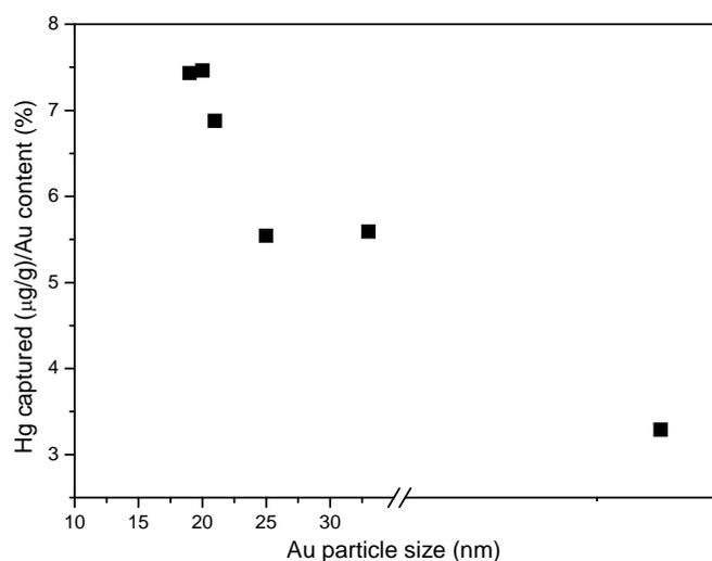
Figure 6. Relationship between Hg captured by the sorbents and the amount of Au and its particle size
