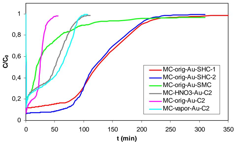
Figure 5. Mercury breakthrough curves for the sorbent.
