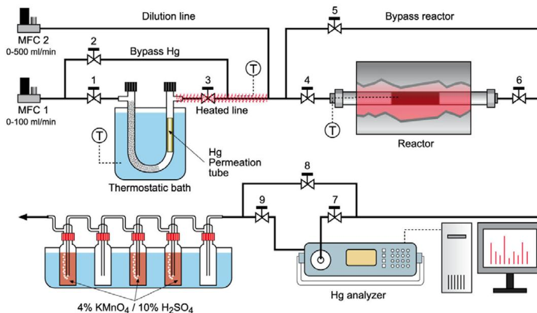
Figure 1. Experimental installation for Hg retention tests.
