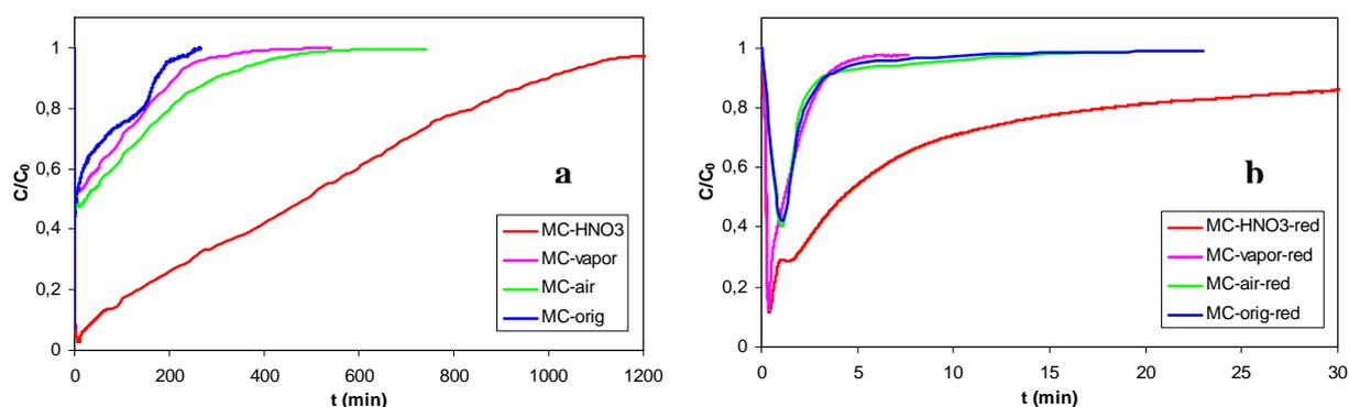
Figure 3. Mercury breakthrough curves for the supports (as prepared and reduced in H<sub>2</sub>/Ar)
