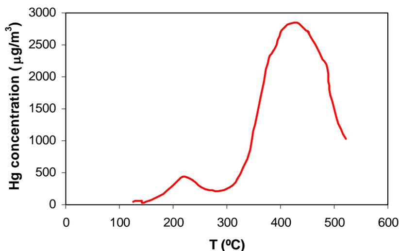
Figure 4 . Hg temperature programmed desorption for exhausted support MC-HNO<sub>3</sub>.
